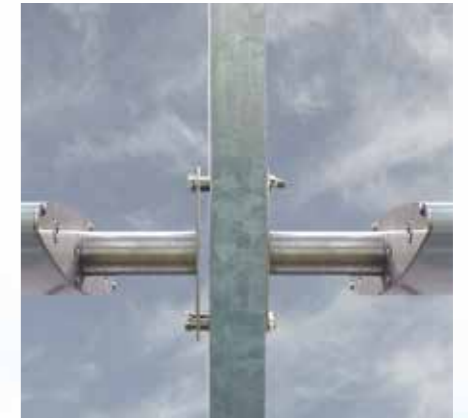
▲ Parallel offset fixing bracket. A detailed view of an 90° parallel offset fixing bracket attaching a CS Airfoil® AF 270F blade onto a vertical support segment is illustrated above. The brackets are screwed directly onto the end of the blade thanks to the special screw channels incorporated into the extrusion. The bracket-blade unit is then fixed with bolts onto the support segment. The availability of parallel off-set fixing brackets and compound angle fixing brackets in a wide variety of angles cater for an unlimited range of design possibilities and adapt to virtually any project specifications.
